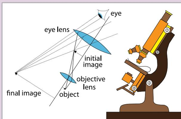
**Figure 2.** Lens/ray diagram that shows how a compound microscope produces an enlarged, but inverted, image of the object. Source: school physics.co.uk. URL: <http://www.schoolphysics.co.uk/age16-19/Optics/Optical%20instruments/text/Microscope/index.html>.
